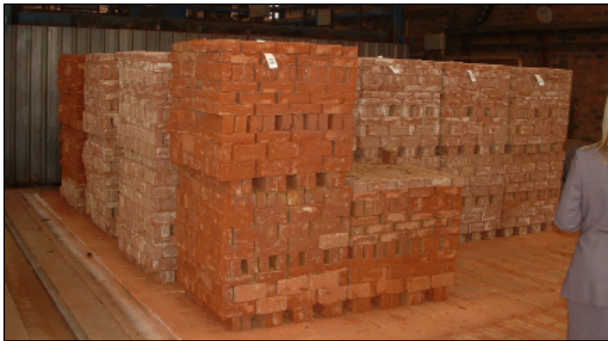
Figure 2. Hearth setting pattern for the moving hood kiln used in the trials.
